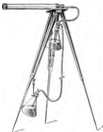
37.—Apparatus for counting microbes in the air.
